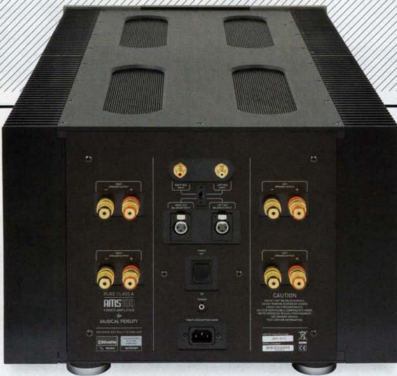
ABOVE: You may select between single-ended and balanced line inputs but – take care – the 4mm speaker outlets are bridged so never connect negative to ground...
